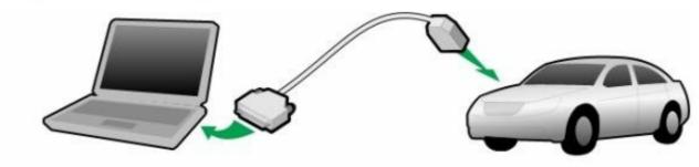
PC Running the Application Using CANCardX for Vehicle Communication
